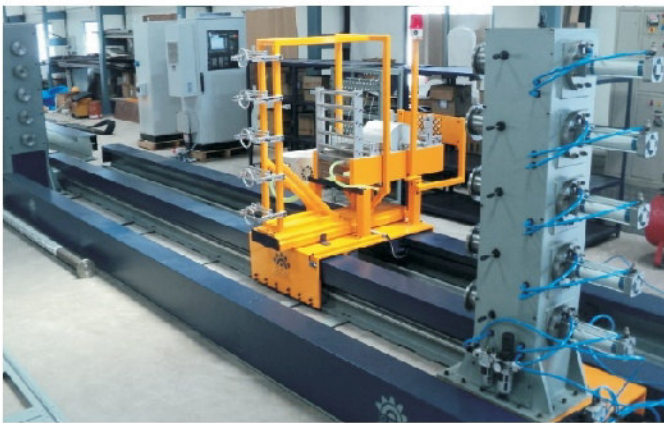
5 Spindle Pipe Winder With Pneumatic Locking, USA
